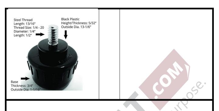
1/4 – 20 thread automatic self adjusting glide that permanently eliminates table wobble. Automatically adjusts each time the table is moved. 12/pk.
